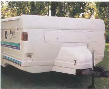
ABS Front Cap has Storage Compartment above body-integrated Bottle Cover
