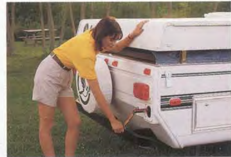
Front and Rear End Caps are made of good-looking, hard-wearing, dent-resistant ABS; Roof Lifter-system Crank is positioned at a comfortable height
