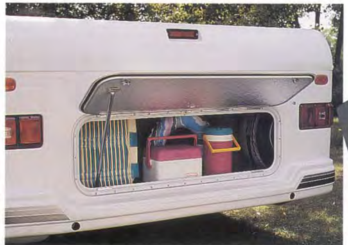
ABS Rear Cap has Full-width Storage Compartment with Spare Wheel
