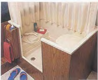
Bathroom features shower, hot & cold faucets, dressing-area curtains, cassette porta-potti, holding tank, water heater, demand water pump, and 20-amp converter
