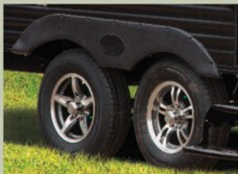
Tandem axles enhance stability
