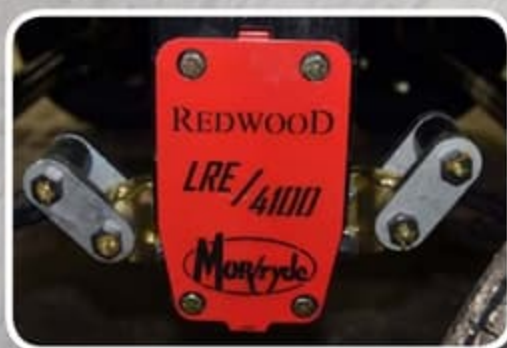
MORyde LRE 4100 Suspension System w/ 17.5" H Range Tires & 8K Axles
