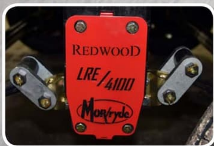
MORryde LRE 4100 Suspension System w/ 17.5" H Range Tires & 8K Axles
